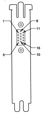
The following table shows the signals and corresponding pin numbers for the 15-pin analog video connector.
